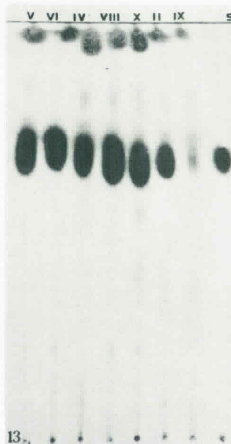
Fig. 13. Chromatogram showing separation of asiaticoside in the leaf extracts of different ecotypes of C. asiatica \times 0.55 (approx.). S = Authentic sample of asiaticoside.
