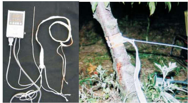
Figure 1. Photograph showing an electric ribbon heater (left) that was used to heat four of the partially ringed peach trunks (R + TH). Photograph on the right shows how the ribbon heater was fitted to heat a tree trunk.
