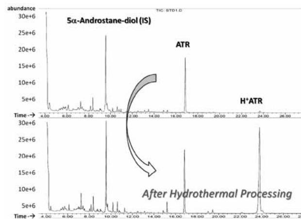
**Figure 3.** Chromatograms of the TMS derivatives of standards. The lower chromatogram shows the acidified and hydrothermally treated ATR (pH 2.3, 98°C) in contrast to the upper one (pH 6.8, 65°C).
