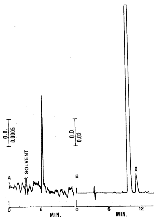
Fig. 3. Liquid chromatograms of GA 3 -ANT. (A) 5 ng; (B) 4 µg; Peak X is impurity. LC conditions: Column, RP C-18, 25 cm; Flow Rate, 0.8 ml/min; Detection, UV at 247 nm; Chart Speed, 0.5 cm/min; Eluting Solvents, (A) MeOH: H 2 O = 80: 20, v/v, (B) MeOH: H 2 O = 70: 30, v/v.
