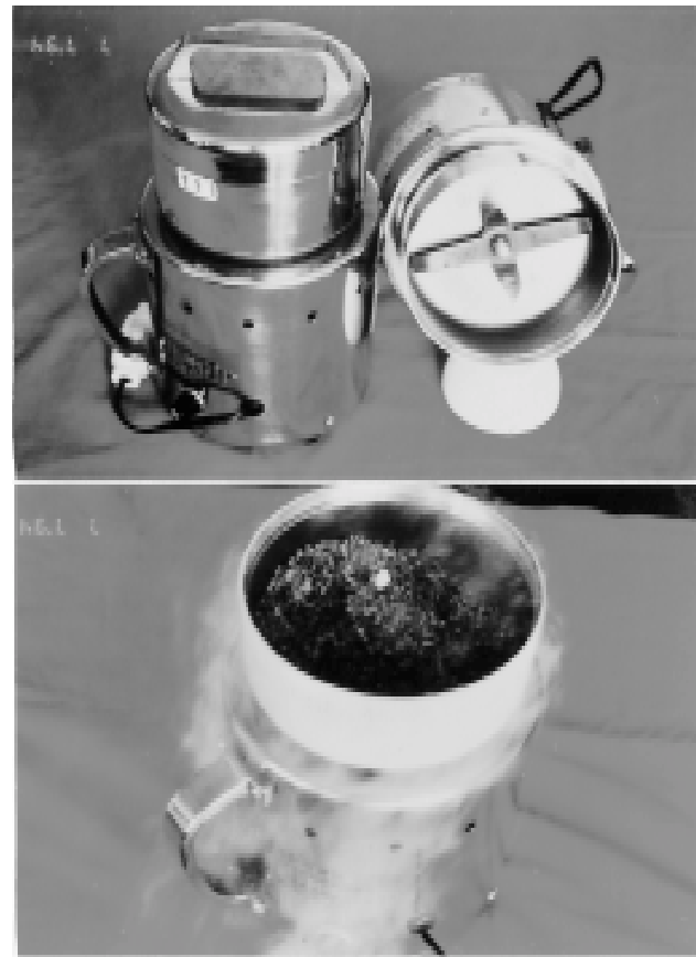
Figure 1. The Chinese herb grinder (Yo-Chi, DM-6) used for the tissue pulverization in the performed tests. Right before the grinding operation, liquid nitrogen was applied to the sample loaded chamber until a thick frosty layer formed on the outer wall (lower picture).
